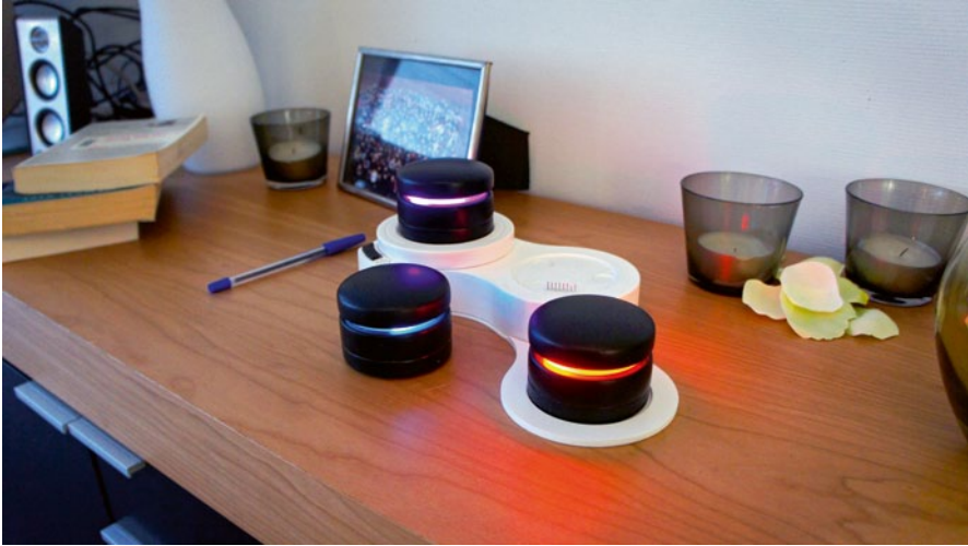
Fig. 4.6 The fully functional final prototype had three messaging tokens and a simplified docking station
